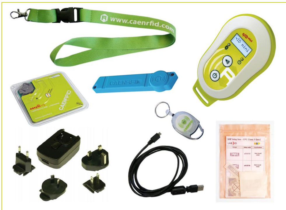
Fig. 1.3: R1170IDK – qIDmini Keyfob Bluetooth UHF RFID Reader Development Kit
